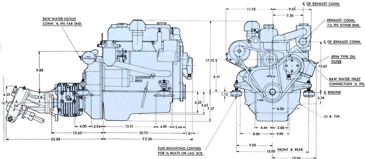
Drawing above shows our **WESTERBEKE Short Profile Sailing Gear**. This compact 2:1 gear has positive neutral for free-wheeling, and instant acting fingertip control. (Use Morse 33C cable or equal). Weight 25 lb. Turns right hand propeller.
